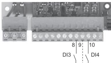
Fig. 6 Digital inputs DI3 and DI4
