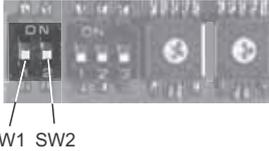
**Fig. 5** Cutting the termination resistor in and out
