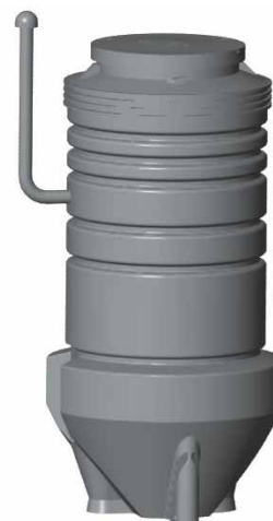
Fig. 15 Pit with vent pipe
